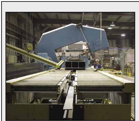
The pultrusion machine shown above (one of the largest in the world), was specially designed by Strongwell to pultrude very large parts, such as Strongwell's 36" x 18" EXTREN DWB® double web beam.
