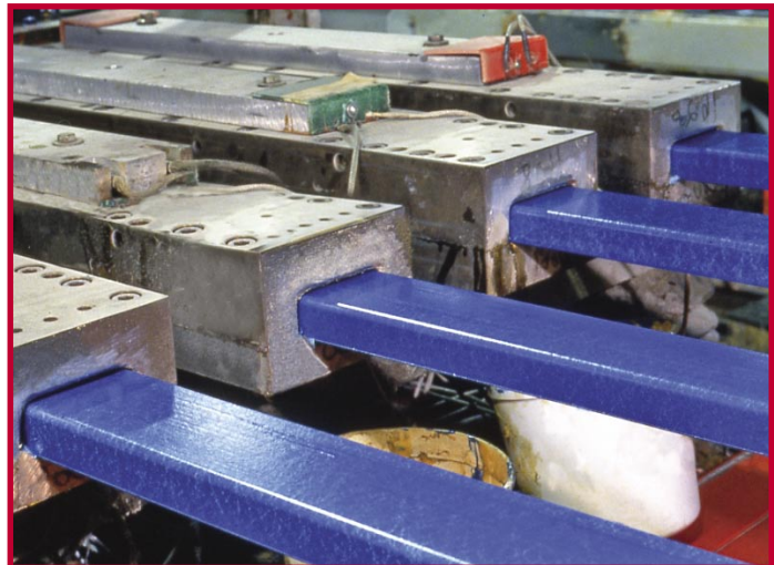
The pultrusion machine shown above (one of the largest in the world), was specially designed by Strongwell to pultrude very large parts, such as Strongwell's 36" x 18" EXTREN DWB® double web beam.
