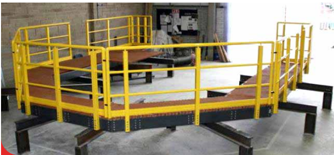
Starboard crane platform fully erected before being disassembled and shipped offshore.
