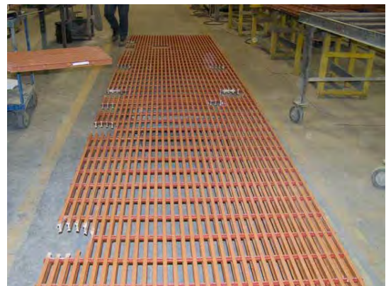
Fabricated panels from Strongwell may (if requested) include adding additional crossrods, penetration plates, pipe sleeves, and identifying areas where additional structure (trimmers) should be added.
