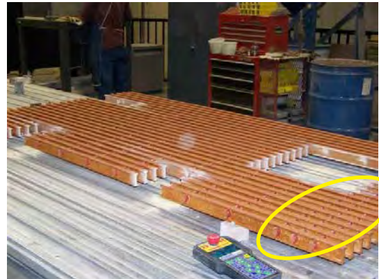
CNC precision cutting from CAD drawings at the Strongwell factory. Note the additional cross rods added to the particular area.
