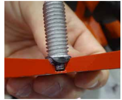
Installed SBT Stud
