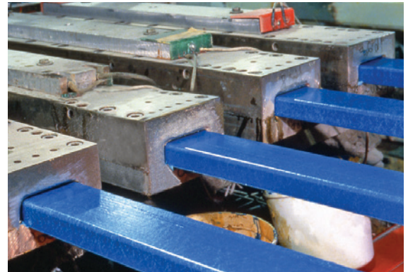
The pultrusion machine shown here (the largest in the world), was specially designed by Strongwell to pultrude very large parts, such as Strongwell's 36" x 18" EXTREN DWB® double web beam.
