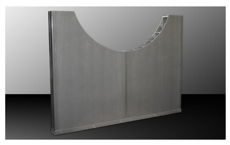
Strongwell has designed and load tested COMPOSOLITE® Pipe Saddles for cooling tower water pipes. These pipe saddles can carry loads up to 25,000 lbs. with a safety factor of 3. Saddles can be manufactured to support pipes from 18" - 60" in diameter.
