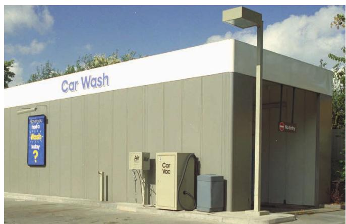
A car wash housing is constructed using COMPOSOLITE® panels, 3-way connectors, and toggles. No internal structure is required. Dimensions are 36' x 16' x 14'-3/4" (11m x 4.88m x 4.29m) high. Low maintenance, ease of construction and an attractive appearance greatly benefited the customer.
