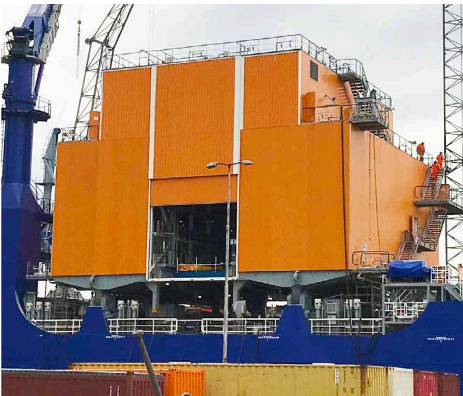
COMPOSOLITE® was outfitted throughout this mobile pipe tower due to its weight savings, particularly important in the lowering of this next generation subsea rock installation vessel's center of gravity.
