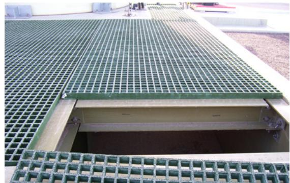
1-1/2" DURAGRATE® was chosen along with EXTREN® wide flange beams as the support structure for a walking surface around equipment at a lift station that houses a wet scrubber for foul air treatment. DURAGRATE® has a high resin content (65%) which provides extended maintenance-free performance.
