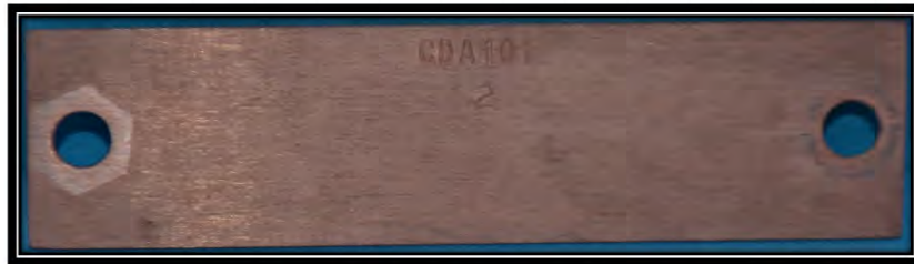
Figure 10: CDA101 after Corrosion Removal
