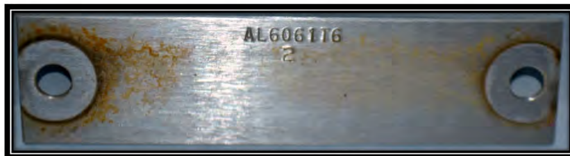
Figure 1: AL6061 T6 Sample prior to Corrosion Removal
