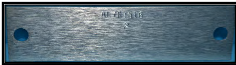
Figure 6: AL7075 T6 after Corrosion Removal
