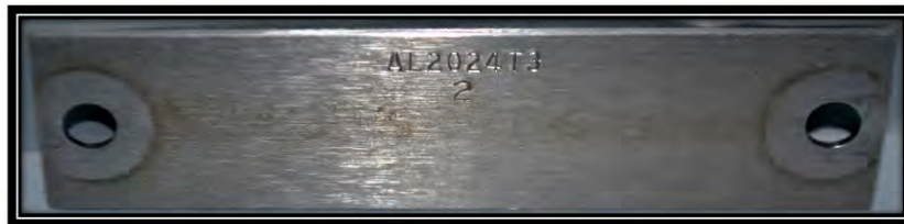
Figure 3: AL2024 T3 Sample prior to Corrosion Removal
