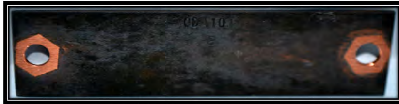
Figure 9: CDA101 Sample prior to Corrosion Removal
