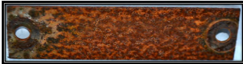
Figure 7: C1010 Sample prior to Corrosion Removal
