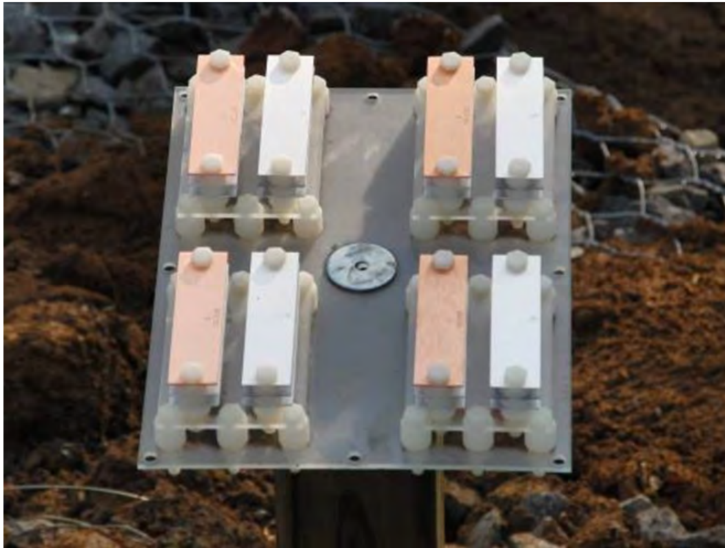
Figure B4. Atmospheric corrosion test rack.
