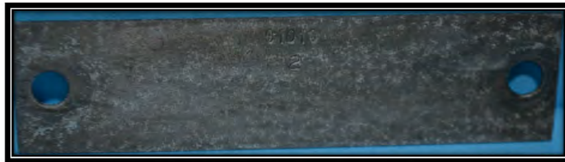
Figure 8: C1010 after Corrosion Removal
