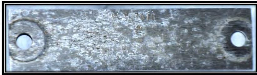
Figure 5: AL7075 T6 Sample prior to Corrosion Removal
