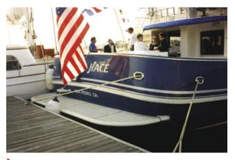
Swim platforms made of fiberglass grating and structural shapes are slip-resistant and will not rot or corrode.
