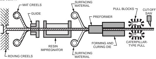
The creels position the reinforcements for subsequent feeding into the guides. The reinforcement must be located properly within the composite and this is the function of the reinforcement guides.
