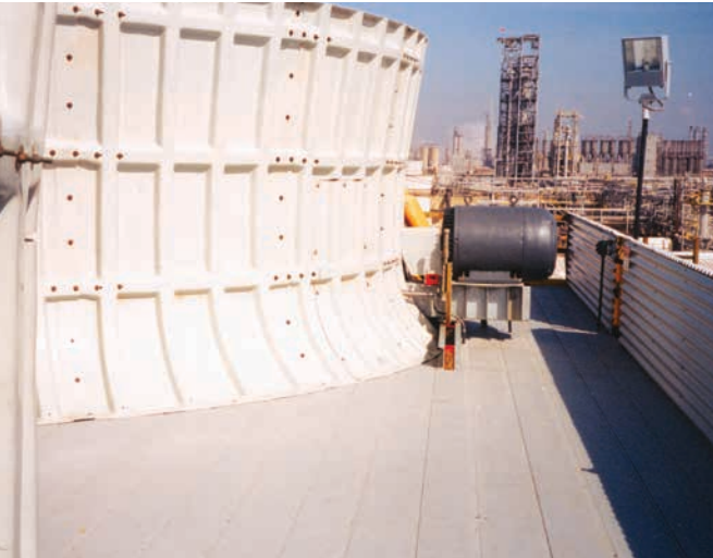
SAFDECK® is used to construct fan decks on cooling towers. The profile height of 1-1/8" is specifically designed to be used as a permanent replacement for rotting plywood on cooling tower fan decks.
