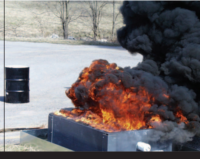
As part of the prototype testing, a burn test was conducted on the COM-POSOLITE oil-containment system. The containment system successfully retained all the oil under the heated conditions.
