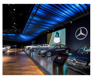
The team at Dimensional Communications Inc. wrestled with the European design, ultimately deciding weight and durability could be achieved by using Strongwell's pultruded FRP at custom lengths ranging from 4 to 20 feet. Each custom FRP component measured 16 inches in height and 2 inches in thickness.
