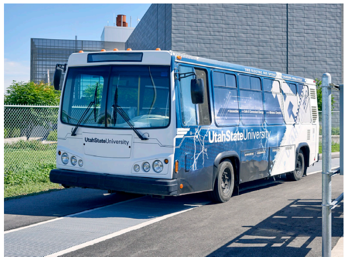
HD-4000 64mm was used as a trench cover to protect wireless electromagnetic charging devices built into the roadway at the Utah State University Electric Vehicle and Roadway research facility in Logan, Utah.
