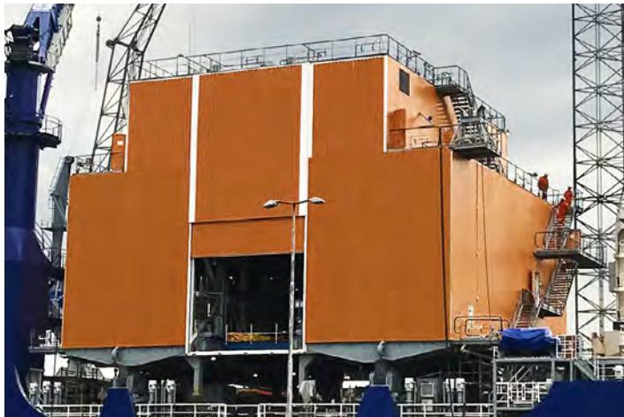
The mobile midship tower measures 20m x 20m x 20m (65' x 65' x 65') in length, width, and height. Since the ship's inception, corrosion and painting were main concerns, as this ship was designed for full automation. When at capacity, it only requires 40 individuals on board for up to 45 continuous days of operation. Composites were utilized not just in the tower, but most of the stair access and landings to the tower were also outfitted with DURAGRID® Phenolic stair treads and grating.
