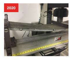
As one of the first generation designs, the panels were assembled with 3/8" FRP rods and polypropylene bushings to achieve proper bar spacing. Today's designs utilize a 3-piece mechanically locked and bonded cross rod design to achieve optimal bearing bar support with peak performance.
