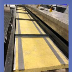
ASTM E84 is the standard test method for assessing the surface burning characteristics of building products to observe the flame spread and developed smoke density. The above photos show the STRONGIRT\* and mineral wool insulation assembly before (top) and after (bottom) testing.
