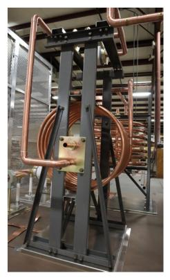
tance was vital due to the station's proximity to the ocean, and so, like most of Kintronic's systems, Strongwell FRP was used for many of the structural components.
