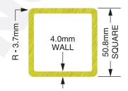
$\begin{array}{lll} A & = & 742.5 mm^2 \\ S & = & 1.077 \text{ x } 10^4 \text{ mm}^3 \\ I & = & 2.735 \text{ x } 10^5 \text{ mm}^4 \\ ^*E & = & 25,500 \text{ N/mm}^2 \\ WT & = & 1.41 \text{ kg/lin. m} \\ ^*E & = & \text{Flexural modulus full strength} \end{array}$
