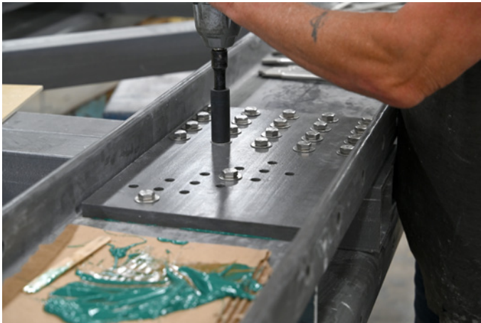
Connections above are bolted plus bonded with adhesive.
