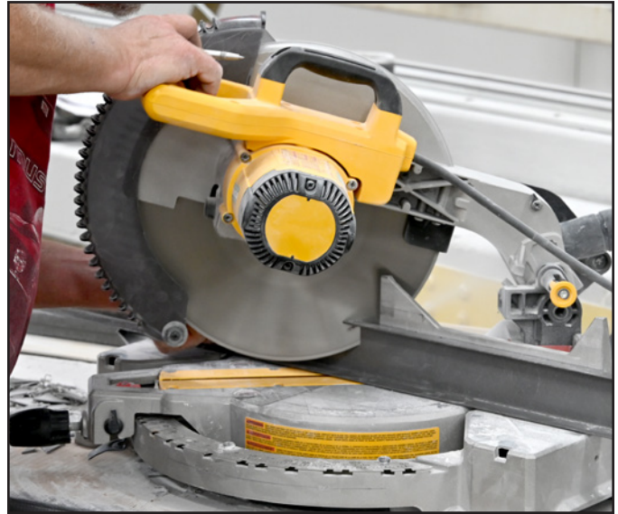
Miter cutting with a miter saw (circular) and diamond grit blade.
