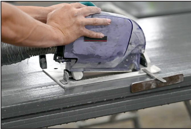
Straight line sawing with circular saw and guide.
