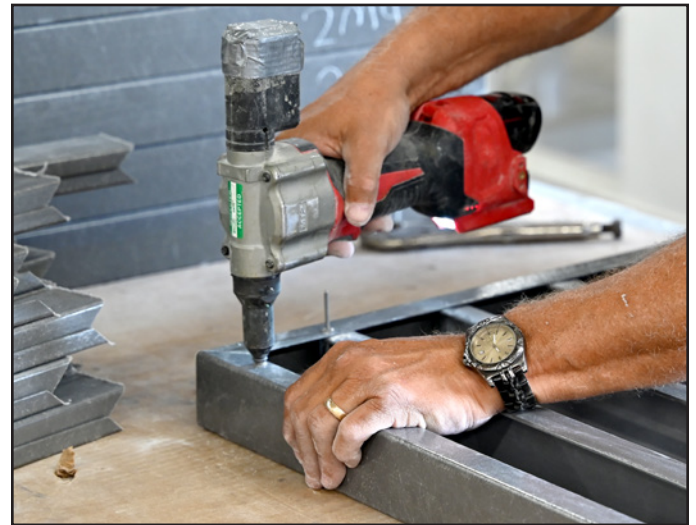
Riveting is a very effective joining method in many applications.
